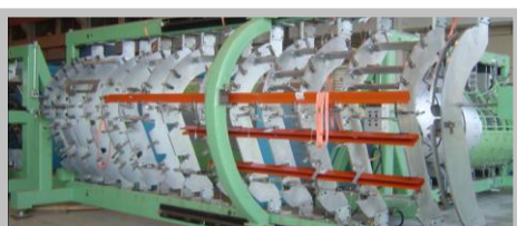
Above, the beginning of the central fuselage sub-assembly.
