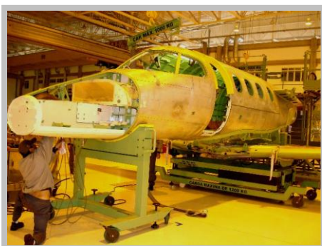
Wing-fuselage mating in Gavião Peixoto, Brazil.
