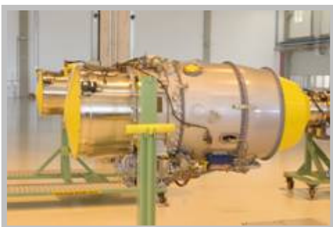
Phenom 300 engines being prepared for installation.
