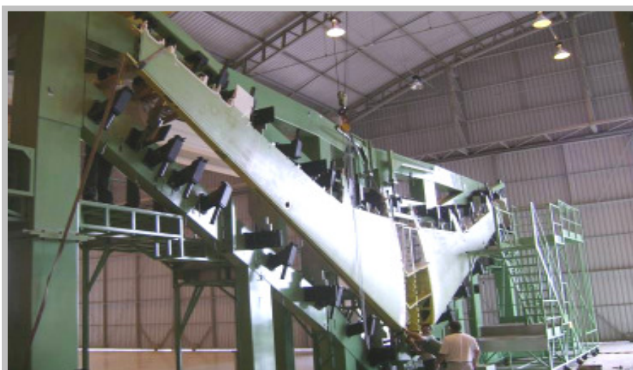
The Phenom 300 wing in production at Botucatu facility.
