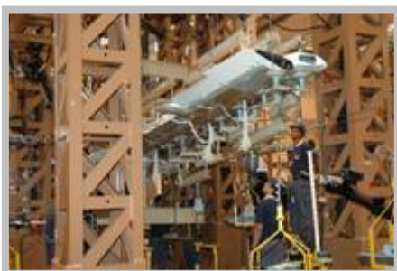
The Phenom 100 wing during overload test
